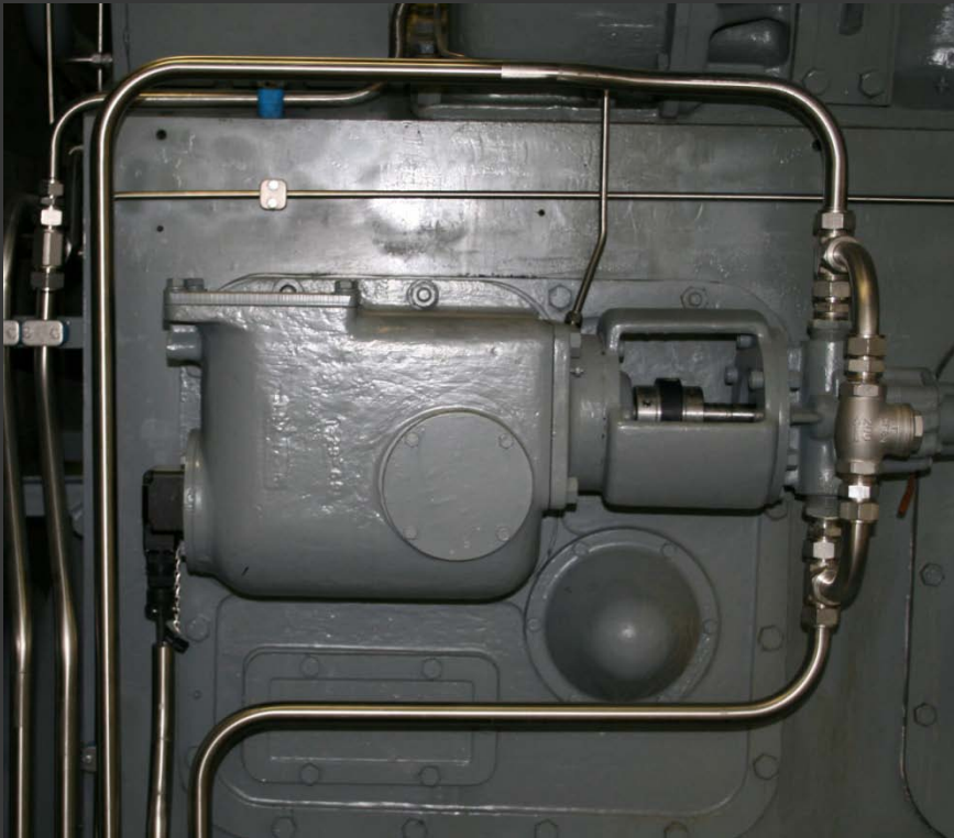
Encoder mounted near original governor location
